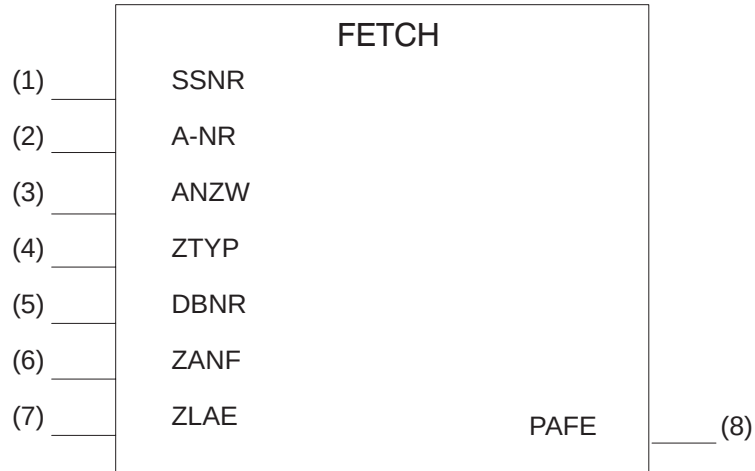
Figure 4-5 FETCH Function Block (FB 122)
